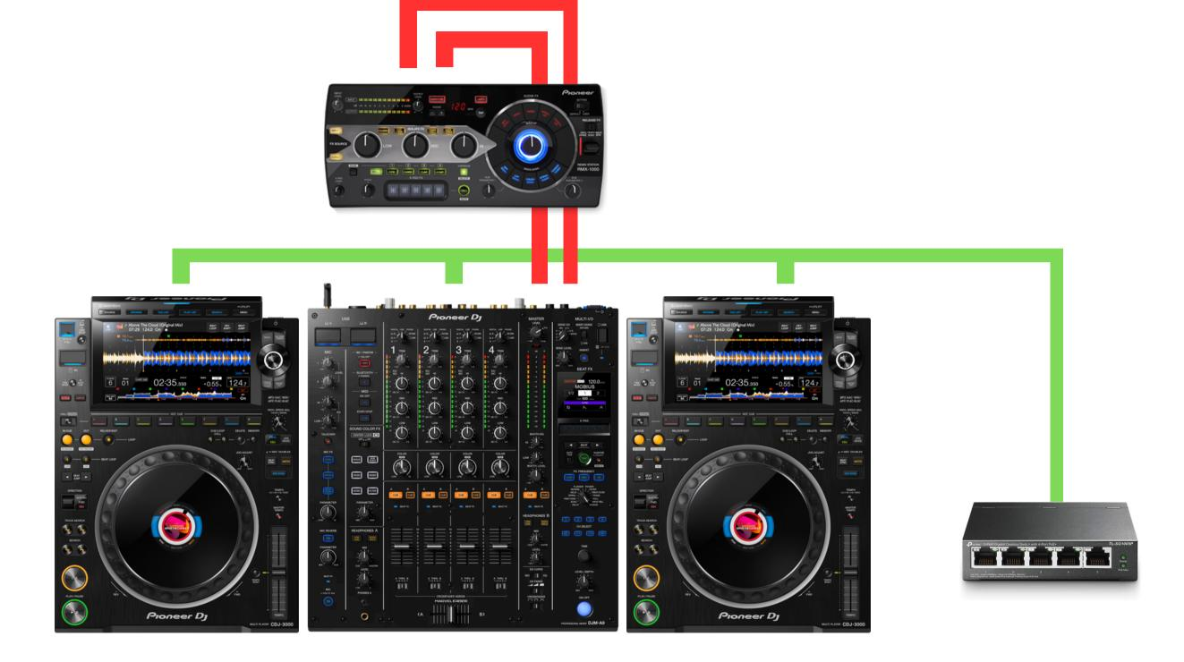
Red Lines refer to TRS cables which should be connected in the following order 'MIXER SEND' - 'IN RMX 1000' - 'OUT RMX 1000' - 'MIXER RETURN'
