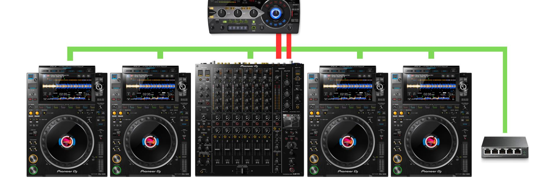
Red Lines refer to TRS cables which should be connected in the following order 'MIXER SEND' - 'IN RMX 1000' - 'OUT RMX 1000' - 'MIXER RETURN'
