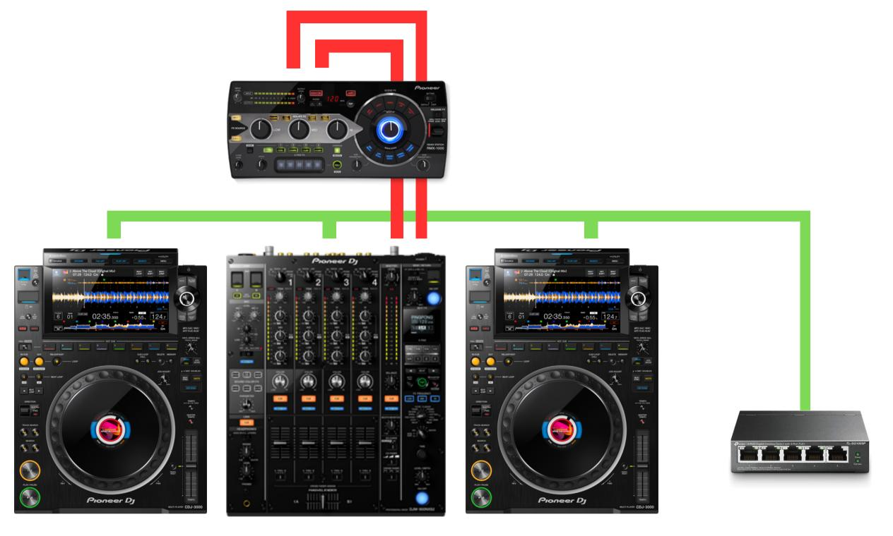
Red Lines refer to TRS cables which should be connected in the following order 'MIXER SEND' - 'IN RMX 1000' - 'OUT RMX 1000' - 'MIXER RETURN'
